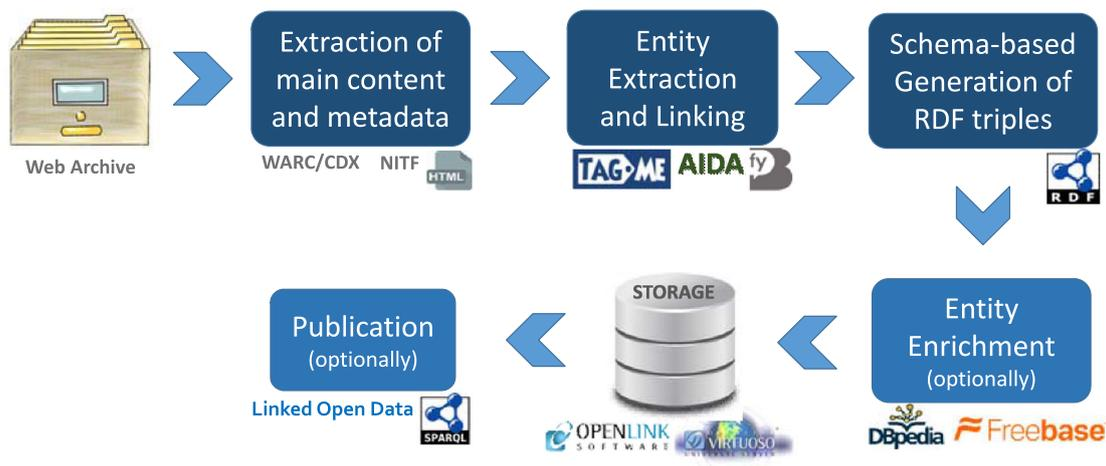
Fig. 4 The process of constructing a semantic layer
